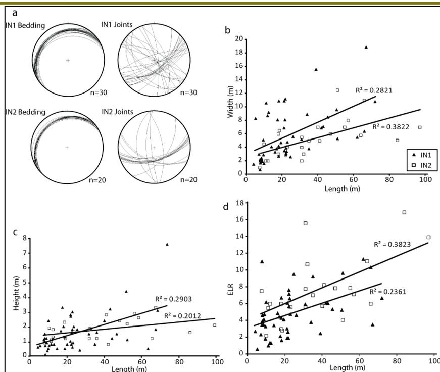
These figures present data from measurements taken of bedrock bedforms in West Greenland. Stereonets visually represent the bedrock joint and bedding plane directions in host bedrock. The graphs display a comparison of two data sets from each site. They represent two very different populations with regard to their height vs length, but in other parameters are less easily differentiated between.
